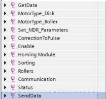
The **Get Data** parts reads out the data from the ProfiNET Device with the given Hardware Identifier
