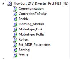
The  $MotorType_Disk$  part scales the speed values from the disk from 0-100% to pulses to send to the controller
