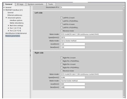
The speed and acceleration can be adapted to the application of the diverters. These settings are the settings that the controller uses after a communication fault.
