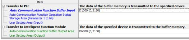
This means that the data configured in de Function Buffer Input is stored from PLC-address D1000 till address D3150 (these are the data read from the Conveylinx modules). The data configured in the Function Buffer Output is stored from PLC-address D6000 till address D8150 (these are the data that is written to the Conveylinx modules).
