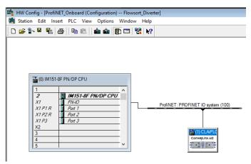
Now the system integrator can give the module an ProfiNET name and IP-adress.
