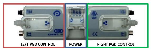
We recommend setting the Conveylinx-Ai2 controller in Full PLC mode via the EasyRoll program. This gives you the advantage that the controller works completely as an IO-module and full control can be done by the PLC. The setting for this mode can also be found in the developer manual of the manufacturer.
