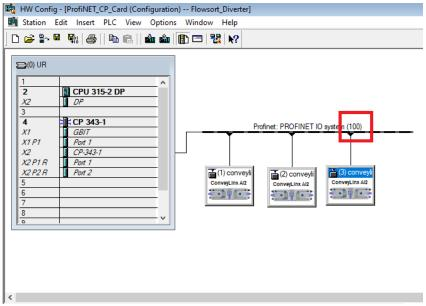
In this example the CPLADDR is **W#16#100**. Use Mode **B#16#0**. The LEN parameter depends on the number of Modules needs to be read out. 1 diverter needs 64 bytes, in this example 3 diverters are configured so 3x64 = 192 bytes. The Data area for the data of the diverters is put at the RECV IO from the function block. This data area needs to be linked to the Flowsort Function block.
