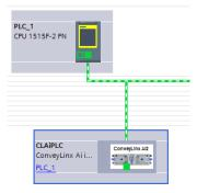
Now the system integrator can give the module an ProfiNET name and IP-adress.
