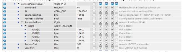
The **interfaceID** is the hardware identifier of the IE-Interface of the configured PLC. The **ID** should be an unique ID for every connection. The **ConnectionType** should be 11 (HEX: 0B). The **ActiveEstablished** should be TRUE. In the **ADDR** the IP-Adress should be set in this example: 192.168.21.182 (HEX: C0,A8,15,B6). **The RemotePort** should be 502 and the **LocalPort** should be 0.
