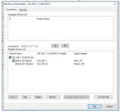
As Originator Variable select the Tag sets that are registered. After the device has been added and integrated, the configuration is necessary to be downloaded.
