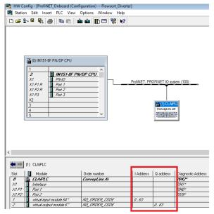
In this example are the input and output start address 0. The "LADDR\_Input" and the "LADDR\_Output" needs to be linked with these start addresses in hexadecimal format. (0 Decimal = 0 HEX but 100 decimal = 64 HEX.)
