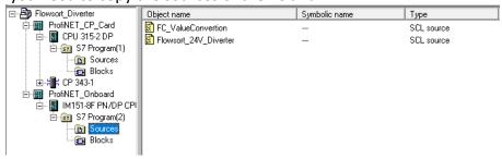
After the copy you need to open and compile first the FC and then FB. When all this is finished without error's there is generated a FC and FB in the Blocks folder.
