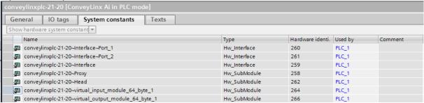
The conv(.....)~virtual\_input\_module\_64\_byte\_1 must be linked to the "Hardware identifier Input" and the conv(.....)~virtual\_output\_module\_64\_byte\_1 must be linked to the "Hardware identifier Output". The linking can be done by selecting the tag and dragging it to the input of the function block you want to link this module to. It can also be done by just typing the number which is in the hardware identifier column at the input of the function block.
