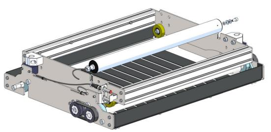
Do not forget to mount the spacer on the M8 screw!
